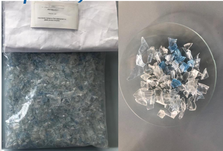
PET flakes (beginning of process)
